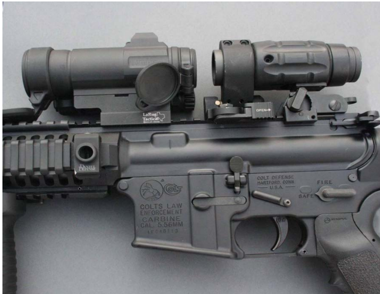
Figure 5. Aimpoint 3 x magnifier mounted behind current M68 CCO. Source: Photograph by author.
