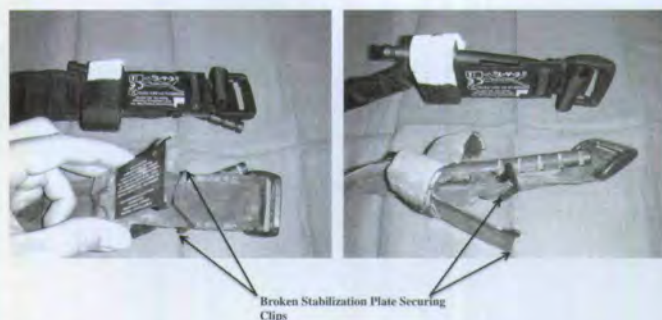
FIGURE 2. Images of Afghanistan-exposed CATs that broke at the stabilization plate.
