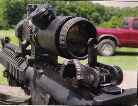
Another advantage of the IOR Valdada Pit Bull is that the BUIS (Back Up Iron Sights) Thompson's Colt LE6940 may be used through it.
