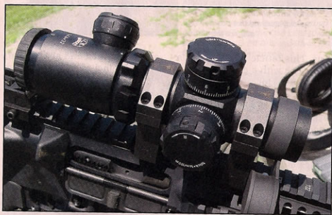
This side view of the mounted Pit Bull shows how carefully the rings must be positioned not to bind the magnification adjustment ring.
