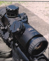
Top view of the Pit Bull shows the elevation dial atop the scope, windage dial on the right, and illumination dial at the bottom. Note the white dot and clearly marked OFF position for the illumination dial. This is very helpful in making sure the illuminated reticle is turned off to avoid running the battery down.
